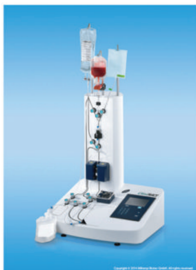
Figure 1. CliniMACS devices. (A) CliniMACS Plus Cell Separation System is a first-generation, semi-automated cell separation system based on MACS® Technology for the development of GMP-compliant manufacturing processes for cellular products. It enables the operator to perform clinical-scale magnetic enrichment of target cells or depletion of unwanted cells in a closed and sterile system. It employs user-friendly software that enables automatic collection of separated cells in different collection bags. (B) The second generation CliniMACS Prodigy System is a closed system enabling GMP-compliant manufacturing and reduction in requirements for cleanrooms, thereby helping facilities achieve GMP compliance without the need for dedicated and expensive manufacturing sites. Several standardised and validated magnetic separation processes can be chosen from the instrument's touchscreen-based menu. Processes have already been developed for the isolation of HSC, specific depletion of alloreactive T cells, enrichment of antigen-specific T cells, and the isolation of monocytes for generation of dendritic cells. In addition, the Prodigy provides a flexible programming option to allow for full integration and automation of complex steps within cell manufacturing workflows.
